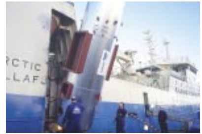
AQ5 composite boiler installed on shrimp trawler by After Sales in Denmark.
